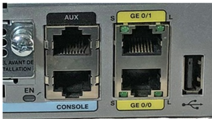
Figure 6-6 Gigabit Ethernet ports on a Cisco router
