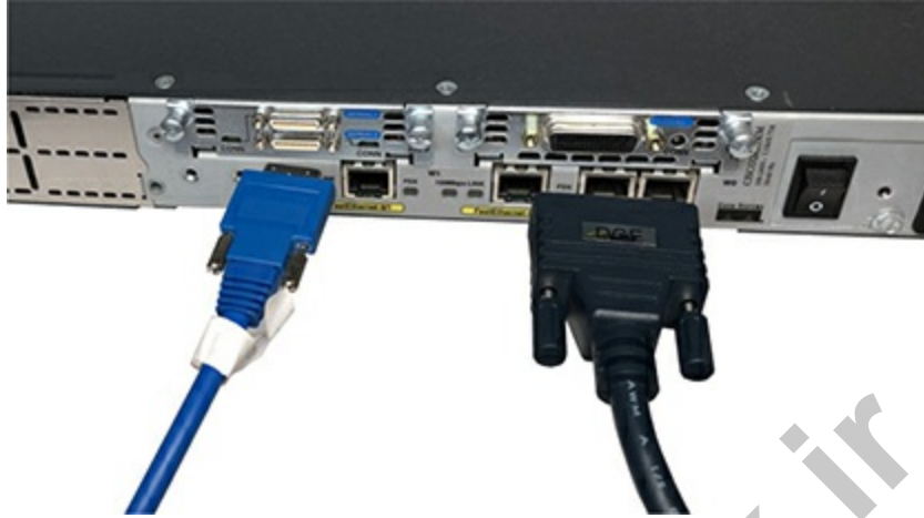
Figure 6-14 Serial cables to connect to the serial ports
