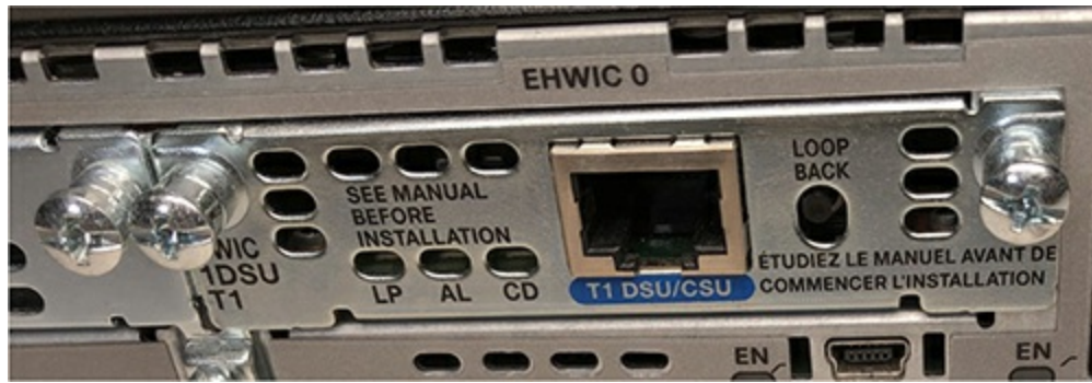
Figure 6-9 An integrated CSU/DSU
