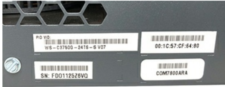
Figure 6-1 Identifying serial number and model number
