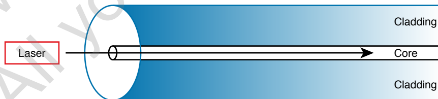
Figure 2-17 Transmission on Single-Mode Fiber with Laser Transmitter
