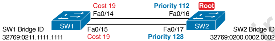
Figure P-2 Topology Required for the Last Two Tiebreakers for Root Port
