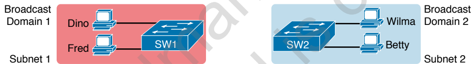
Figure 8-1 Creating Two Broadcast Domains with Two Physical Switches and No VLANs
