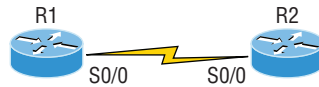
FIGURE 6.6 By looking at R1, the show controllers command reveals that R1 and R2 can't communicate.
