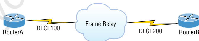
FIGURE 21.20 Frame Relay mappings
